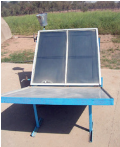
Figure 17. Collector cum storage type solar water heater.
