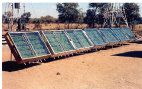
Figure 13. Solar dryer developed by ICAR-CAZRI, Jodhpur.
