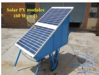
Figure 6. Solar PV sprayer.
