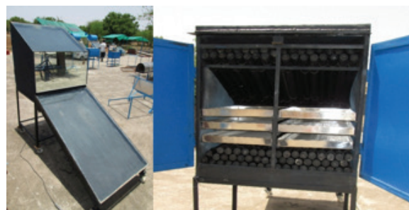
Figure 14. A flat plate absorber with thermal storage natural convective solar crop dryer.
