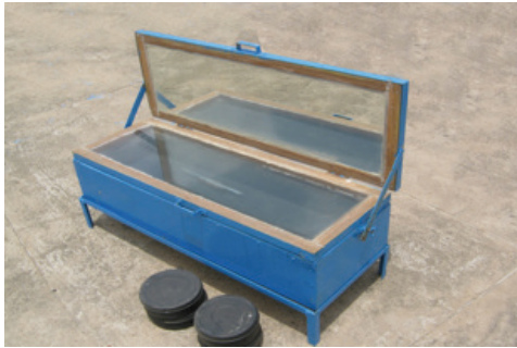
Figure 15. Installation of the non tracking solar cooker.
