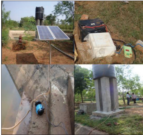
Figure 4. Solar based micro irrigation system for lifting farm pond water.
