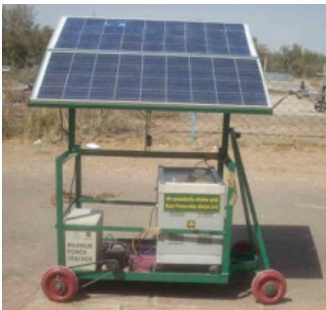
Figure 11. PV mobile unit developed at CAZRI, Jodhpur.
