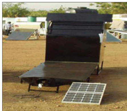
Figure 4. Indirect solar dryer (Rozis, 1995).
